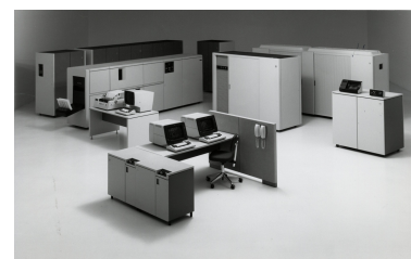
The IBM 3081 mainframe class supercomputer introduced 1980 had 16 MB of RAM and apparently cost around 3–5 million USD at the time. Yes, this whole setup is the computer, including printer, tape drives, terminals, etc. For an interesting personal viewpoint, see https://www.tomshardware.com/picturestory/508-mainframe-computer-history-2.html (Photo: Norsk Teknisk Museum.)
